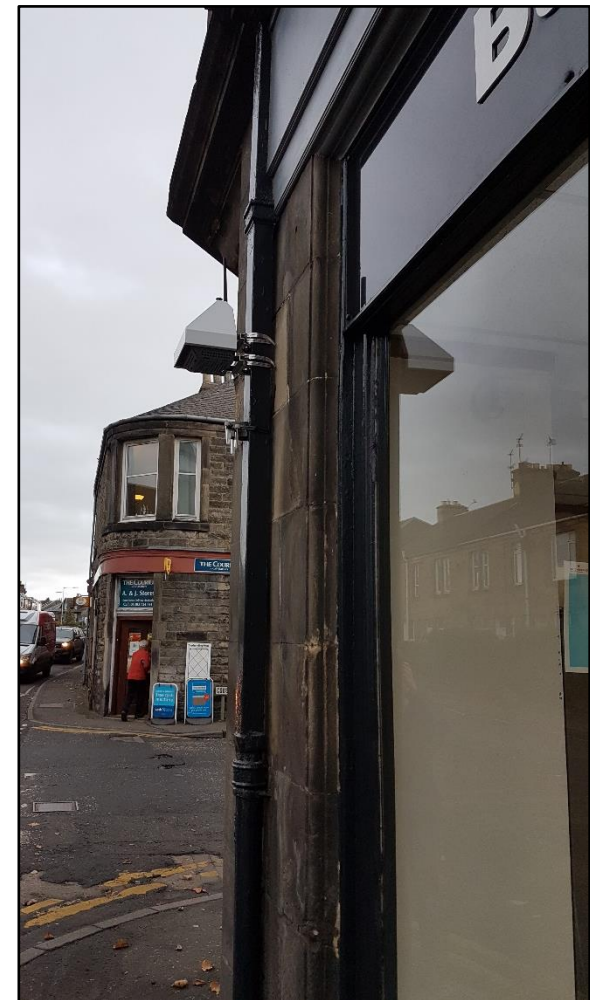
Appin Crescent East AQMesh sensor (co-located with triplicate diffusion Appin Crescent 5A,B & C)
