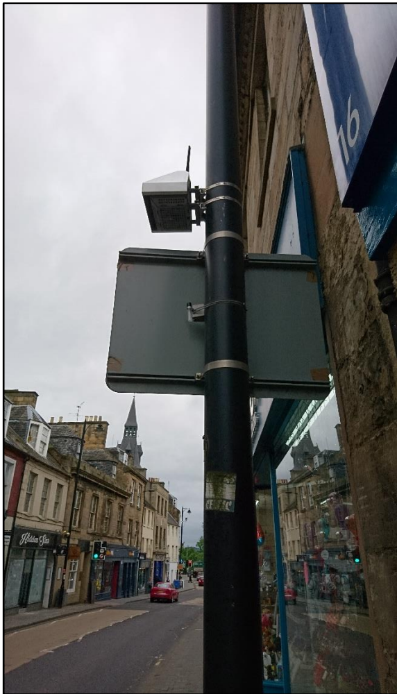
Bonnygate AQMesh sensor (co-located with diffusion tube Bonnygate B4)
