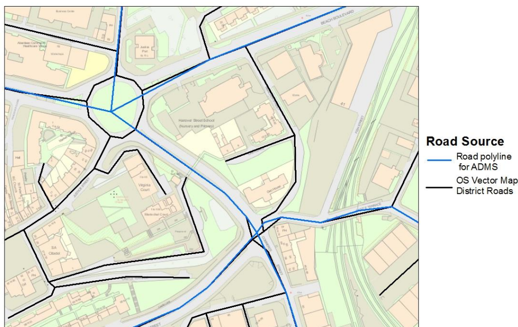
Figure 7: Example of Digitised Roads and modified road layout for ADMS
