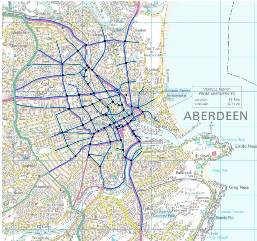
Figure 11: Aberdeen road network generated from city council traffic data. Black dots are count point locations
