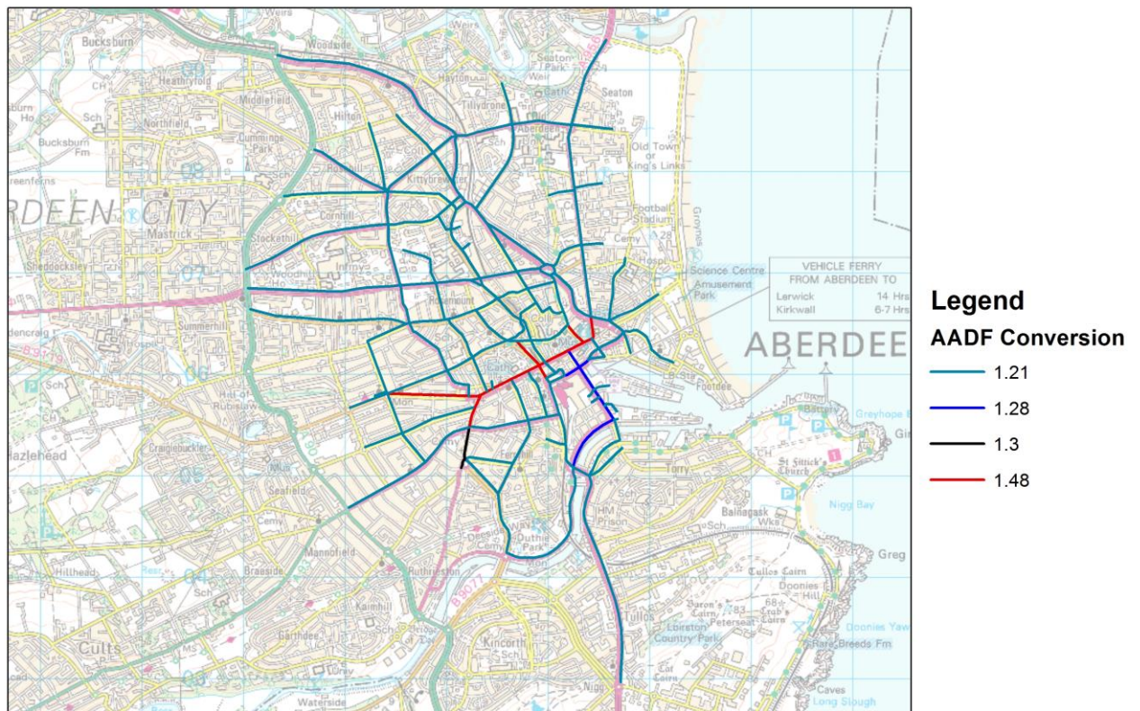
Figure 13: Conversion factors for 12 hour count to AADF for each road section
