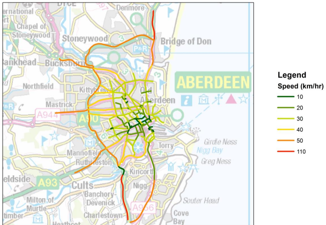
Figure 19: Traffic Speeds used in Aberdeen ADMS-Urban model for each road section
