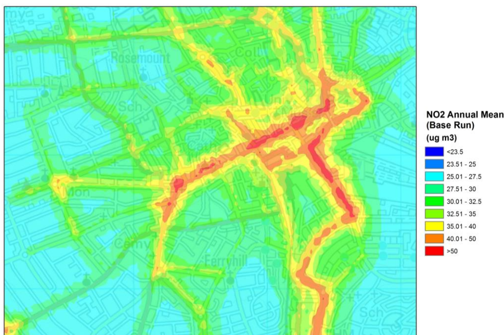
Figure 107: Predicted NO 2 Annual Mean concentration ( \mu\text{g m}^{-3} ) in Aberdeen City Centre (Base Run)
