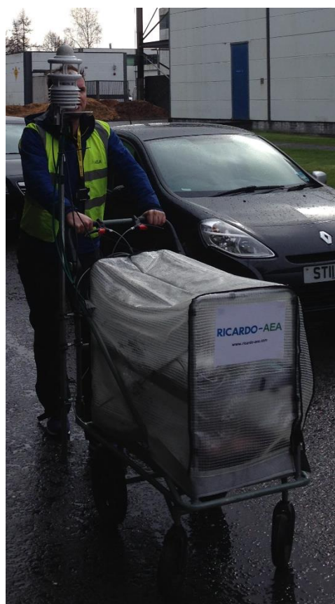
Figure 3-1 a&b: a) Trolley containing air sampling instruments, including Lighthouse IAQ 3016 b) Purpose-built backpack , including Lighthouse IAQ 3016
