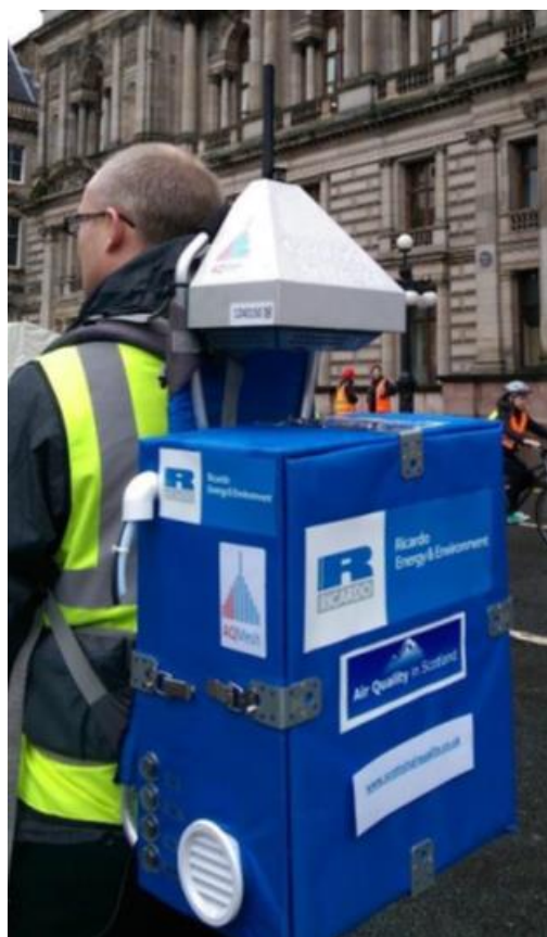
Figure 3-1 a&b: a) Trolley containing air sampling instruments, including Lighthouse IAQ 3016 b) Purpose-built backpack , including Lighthouse IAQ 3016
