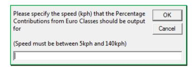
**Note 14:** If a user is running the EFT with the Output % Contributions from Euro Classes Advanced Option, all other EFT outputs selected for the model run will be based upon the speeds entered on the Input Data sheet on a link-by-link basis.
