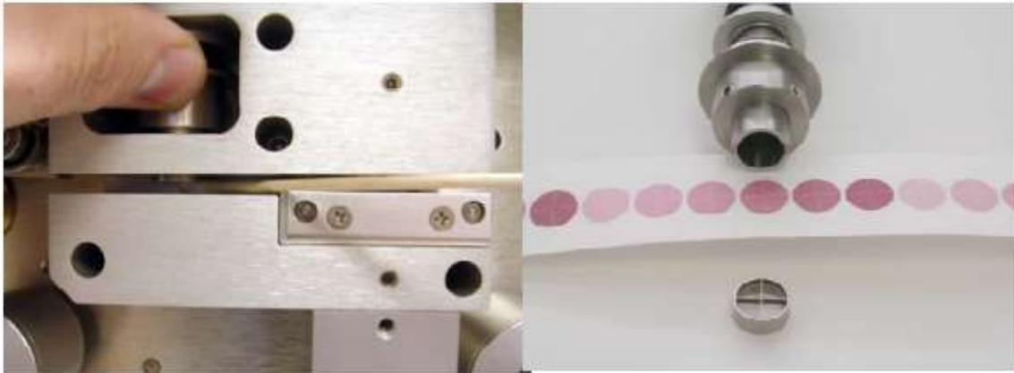
**Figure 21-4** A cotton-tipped applicator and isopropyl alcohol are used to clean the BAM-1020 nozzle and vane (left panel). A view of the nozzle, sampled filter tape, and filter tape support vane are shown in the right panel.
