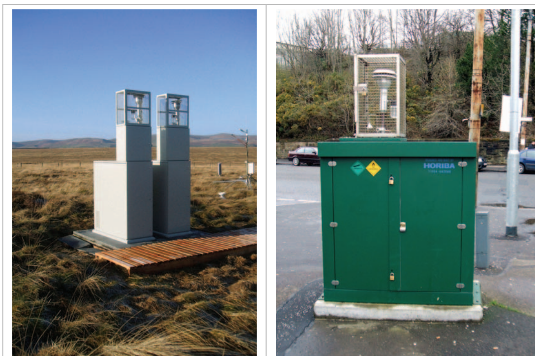
Figure 2 Urban and rural: Glasgow Battlefield Road (right) and Auchencorth Moss (left) automatic air quality monitoring stations
