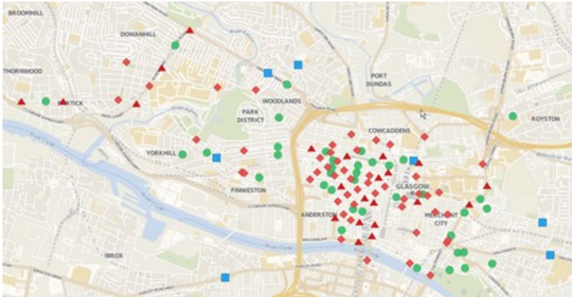
Figure 3 - Example of detailed traffic collection points, including turn counts, 12/24 traffic count locations and ANPR (data collected in Glasgow during winter 2017/18)
