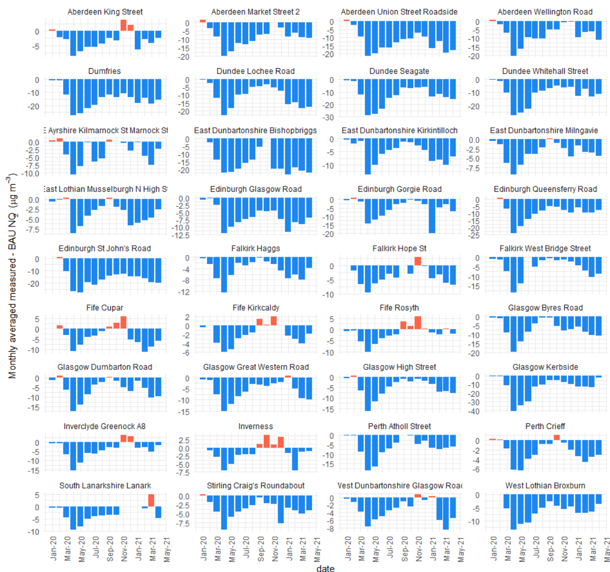
Figure 23 Monthly mean difference in measured and modelled "business as usual" (BAU) concentrations for urban traffic sites. Red bars represent measurements greater than modelled concentrations and blue bars represent measurements lower than modelled concentrations. Note the different scales on the y-axis for each site.
