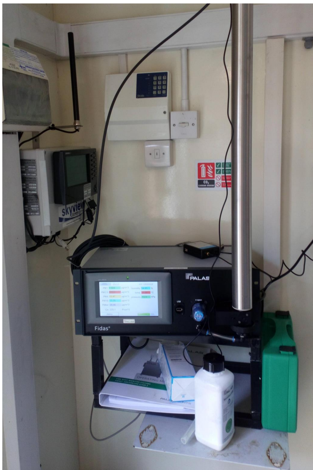
Photo 3 Palas Fidas 200 Combined PM 10+2.5 Analyser at the Grangemouth Zetland Park Site
