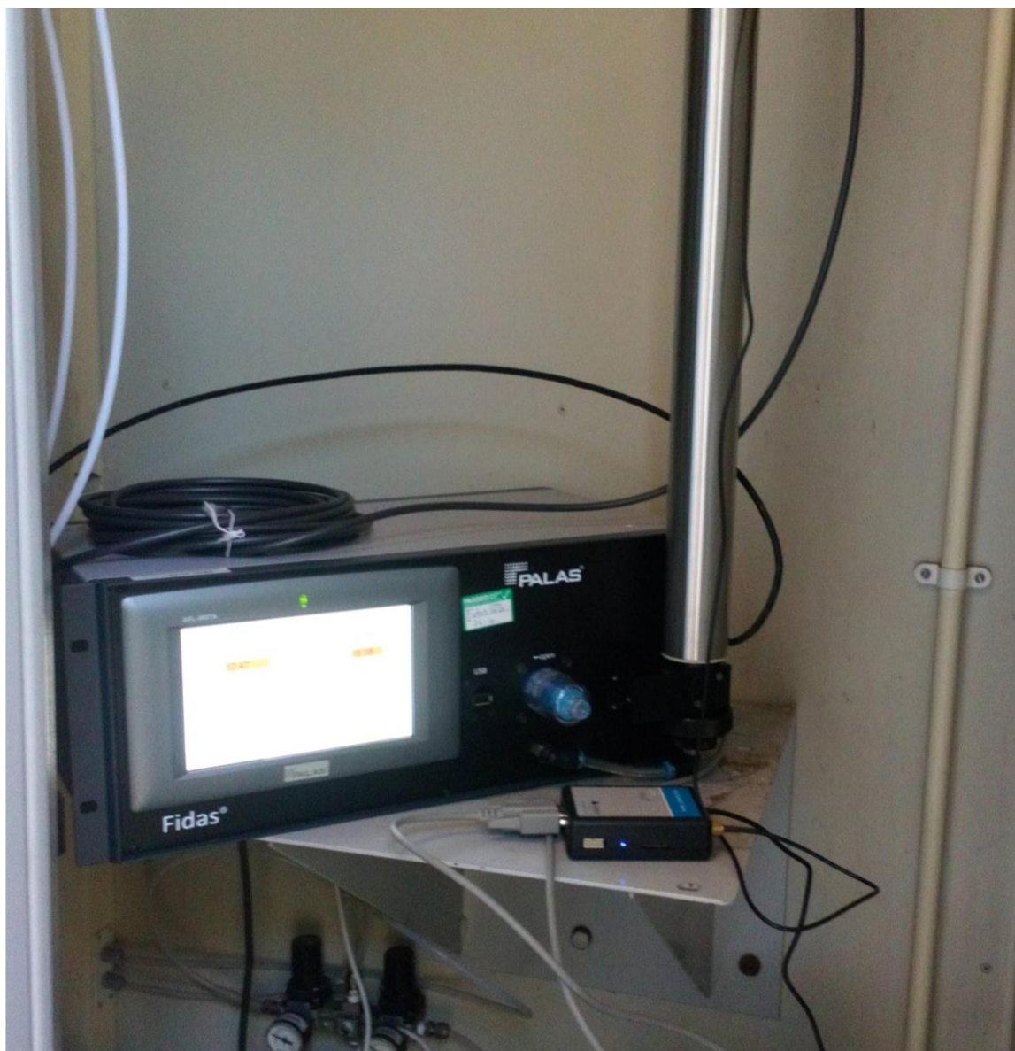
Photo 1 Palas Fidas 200 Combined PM 10+2.5 Analyser at the Falkirk Hope Street Site
