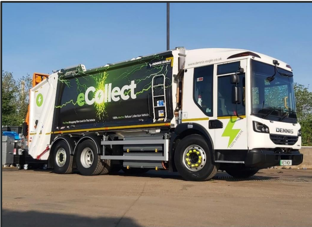
Figure 2-13 Dennis Eagle eCollect refuse collection vehicle recently trialled by Fife Council
