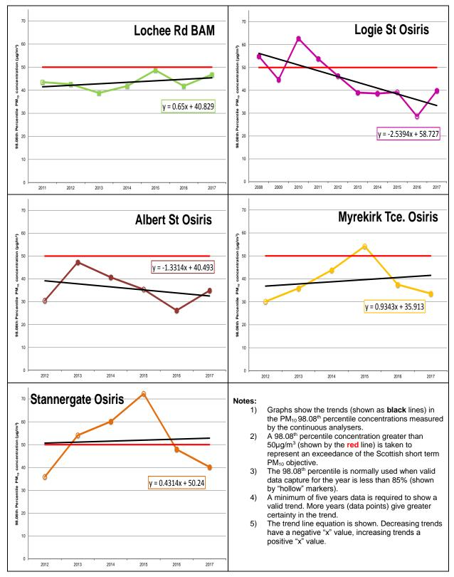
Figure A6.c Trends in 98.08<sup>th</sup> percentile PM<sub>10</sub> concentrations at Automatic monitors
