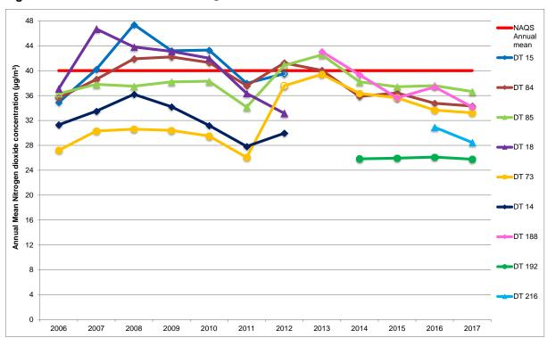
Figure C.21 Overview of Other NO<sub>2</sub> Diffusion Tube Concentrations on Bus Corridor
